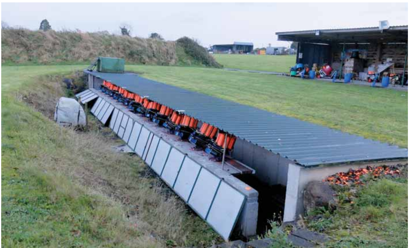
The Olympic trap layout with 15 machines in the line.
