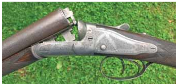
This Rigby back action side-lock 12-bore is made on a Scott action and is typical of the style of the 1880s, when gunmakers were experimenting with new designs. The fine scroll engraving and gothic lettering are very 'Rigby'.
