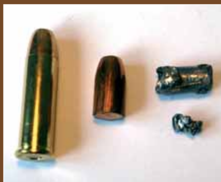
Problem ammunition (L - R) .38 Special round along with the bullet that failed to exit the barrel and lead centre of the round that had to be forcefully cleared
