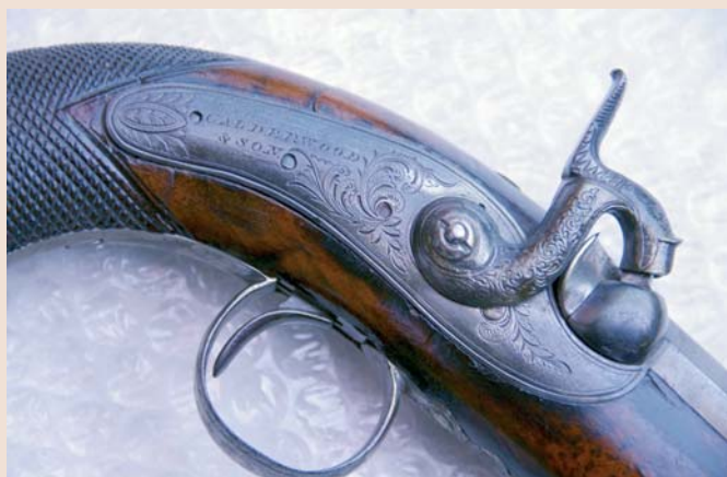
Calderwood & Son Backaction Pistol Lockwork. Reproduction with permission from the collection of Victoria Police.
