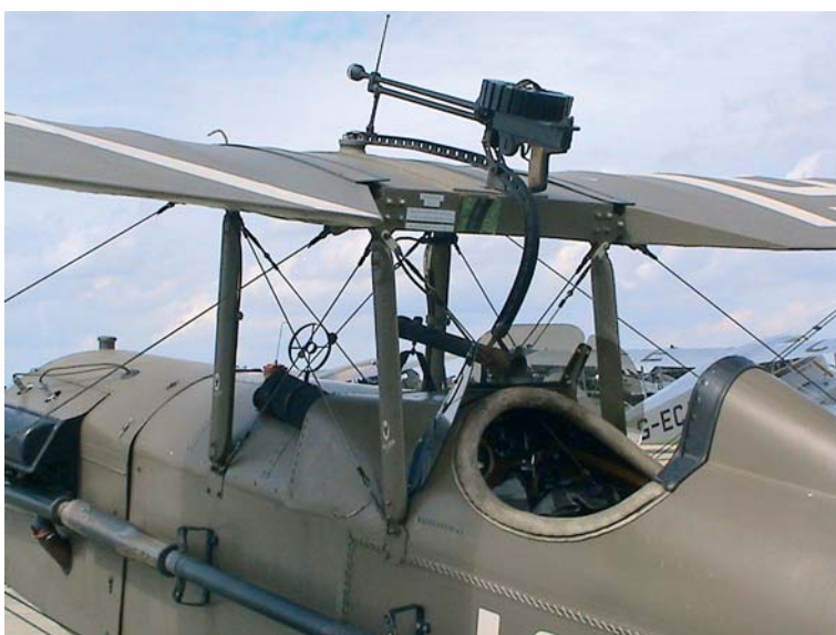
(Left) Lewis Gun in situ - note that it was fired from above the pilot's head.
